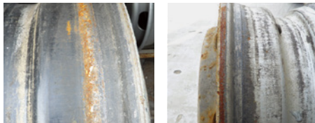
Corroded steel wheel
