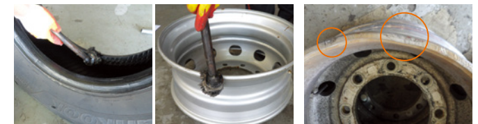
Correctly applied tyre lubricant
