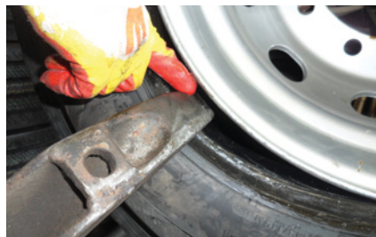
6 The gap between the wheel flange and the hook needs to be just smaller than a finger to fit between. If the gap is too wide or too narrow there is a risk of damage to the wheel flange or tyre bead.
