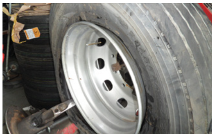
5 Operate the tool arm to pull the hook in the direction of the operator.
