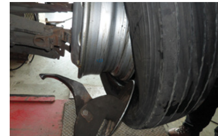
9 Move the tool arm to the opposite side of the bead (not the demounted side) and manipulate the bead disc breaker to further separate the tyre from the wheel.
