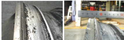
Sharply worn/deformed rim flange
