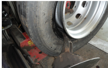
4 Push the hook into the end of the tyre bead and lower it down so that the top of the hook does not come into contact with the wheel.
