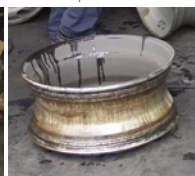
Application of incorrect tyre lubricant
