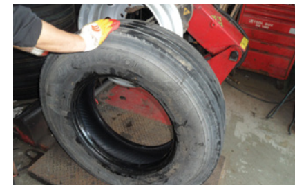
11 Rotate clockwise and to completely separate the tyre from the wheel. * Be careful as the tyre will fall in the direction of the operator.
