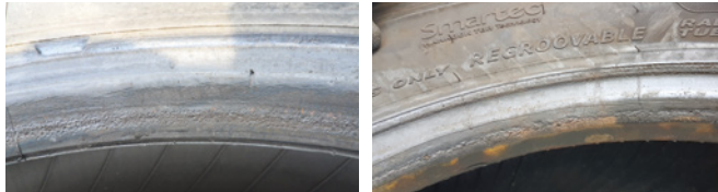
Contaminated bead by corrosion from the steel wheel
