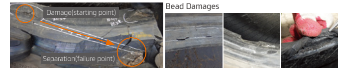
Torn outside bead
