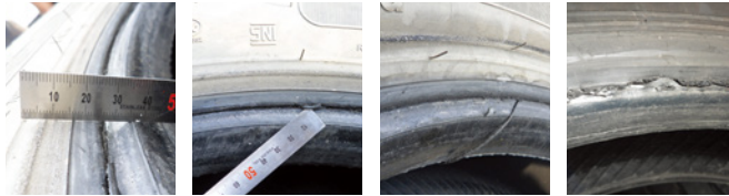
Torn tyre bead
