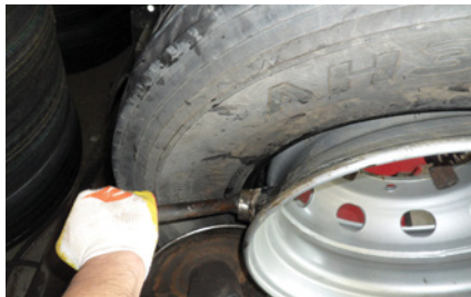
3 Create some space between the tyre and wheel by the bead breaker disc and apply tyre lubricant to the rim flange and tyre bead to prevent tyre damage.
