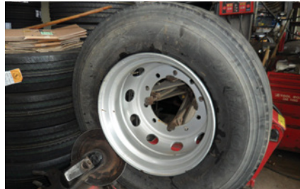
2 Fix the assembly to the automatic machine; using the machine arm locate the bead breaker disc on the drop centre.
