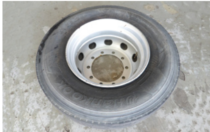
1 Completely remove the air in the tyre.
