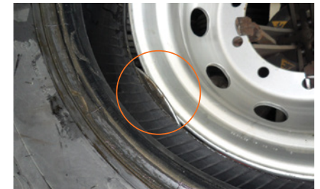
10 Position the bead breaker disc to sit between the rim flange and the tyre bead. The disc should not touch the wheel.
