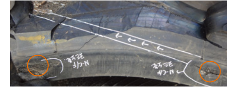
Damage occurred in mounting procedures
