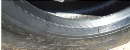
Bead deformation by excessive pressure of automatic machine
