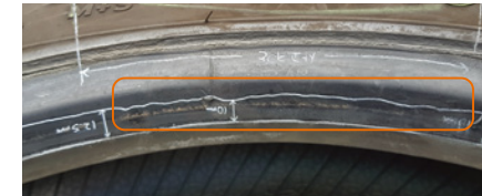
Trace of non-uniform rim fitting (white line)
