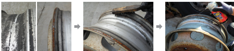
<Contamination on aluminum wheel>
