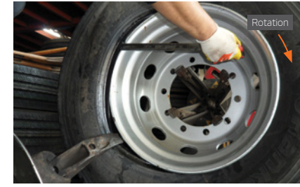
7 Put the lever between the wheel flange and the tyre bead and rotate clockwise.
