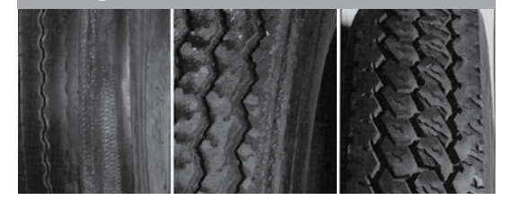
Flat spotting due to locked brakes
